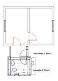
Drawing 10: Different cases of the construction of bathrooms and entrances in Kraljevo
