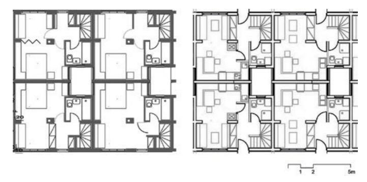
Drawing 43: SOLECO type incremental enlargement house evolving around the kitchen and a bathroom
