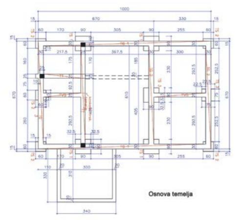
Drawing 40: Project for the foundation that can be one of the core house construction types
