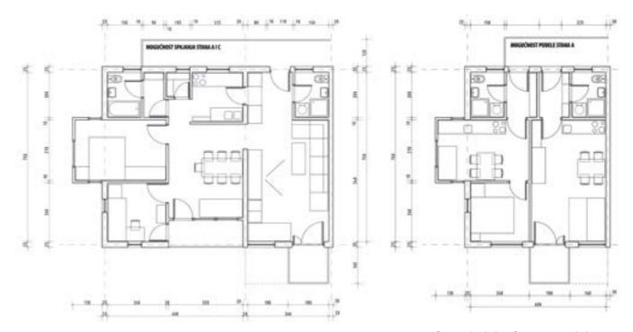
Drawing 21: A plan of apartments with the possibility to divide or attach apartments
