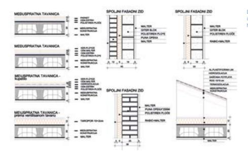
Drawing 13: Details of thermal insulation in the case of a completion of unfinished houses model
