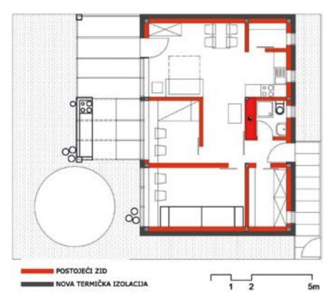
Drawing 14: An example of placing thermal insulation on an unfinished house
