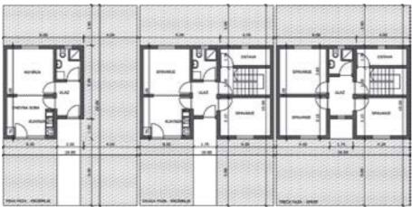
Drawing 8: Construction of an additional room, as an enlargement of the original house
