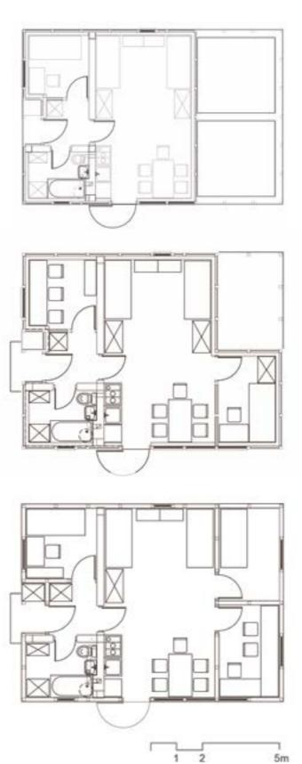
Drawing 42: Project for an incremental enlargement house evolving around the kitchen-bathroom core
