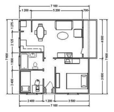
Drawing 28: Prefabricated house - ground surface 60 m<sup>2</sup>
